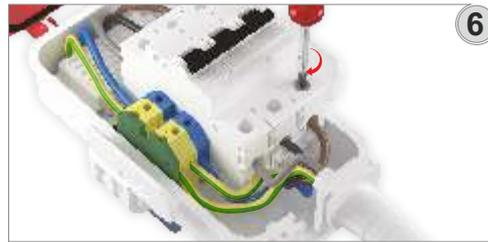
Install the feeder cable at the fuse outlet terminal in the same way. Make sure that the screws are tight.
