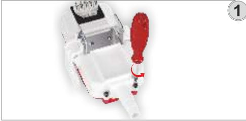
Use 052XZ1-F type cable, (3x2,5mm<sup>2</sup> for single phase, 5x2,5mm<sup>2</sup> for three phase) as required. Turn over the tap-off box and remove the two screws.
