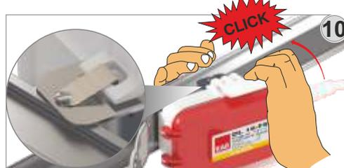
First, connect product earth terminal to busbar plug-in point. Then make sure that other terminals connect to busbar. Finally you should hear "CLICK" sound when you press tap-off box towards busbar.
