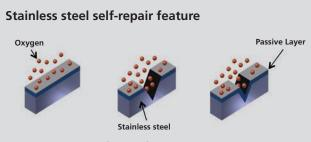
The metallic satin finish of the stainless steel makes itself passive, if a suitable environment is provided, i.e. sufficient oxygen and available rich chromium oxidation.
