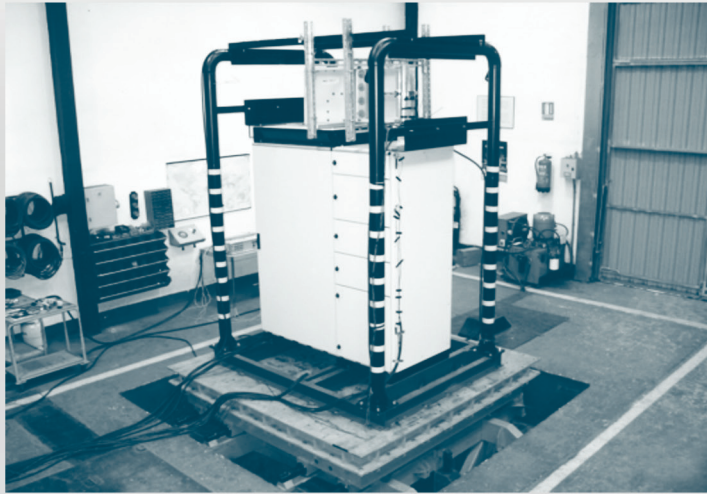
Seismic test in accredited laboratory with busbar connection module for Richter scale 7 and above
