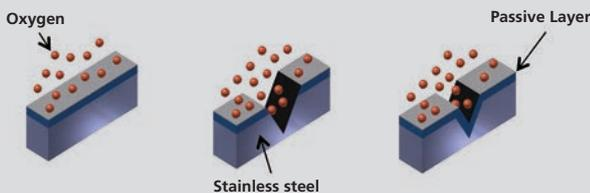
The metallic satin finish of the stainless steel makes itself passive, if a suitable environment is provided, i.e. sufficient oxygen and available rich chromium oxidation.
